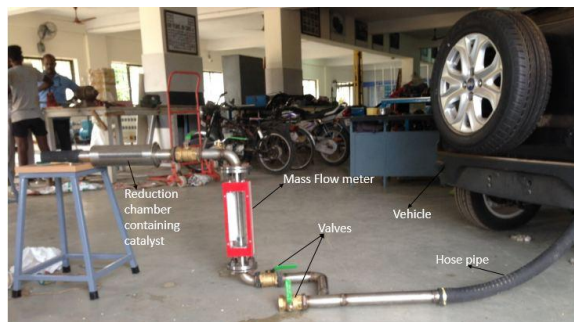
Fig : 12 Vehicle assemble with CO 2 adsorption chamber
