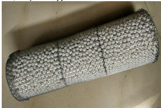
Fig : 10 Wire mesh filled with Catalyst
